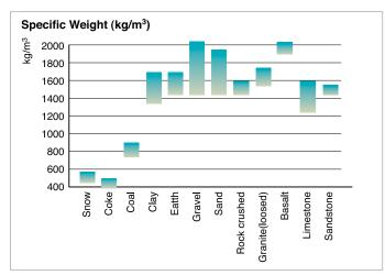
The specific weight of material largely depends on moisture rate, compacting value, The Bucket filling factor depends also of the nature of material, the working conditions percentage of various components etc... This chart is given only for information.
