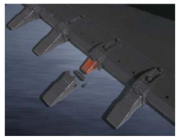
2-Piece Type Tooth(Pin-on+Bolt-on adapter)
