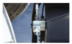
Remote Engine oil & Coolant Drain
