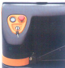
Combination control panel
