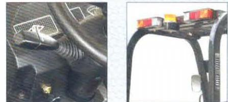
The torque converter models adopt electronic-hydraulic forward-reverse control technology, meaning less effort and less total time used during this often-performed function.
