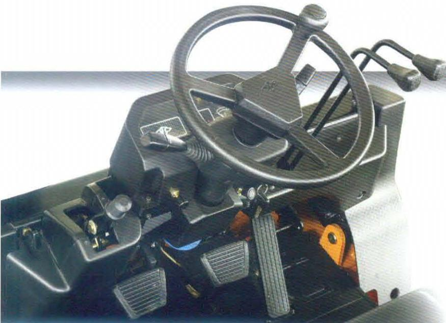
The grease fittings and bushes added around the shaft of control mechanism decreases the force of pedal, that are reduced 30% compared with former truck.
