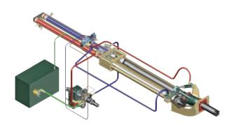
Direct connecting main pump and hydraulic cylinders improve pumping efficiency
