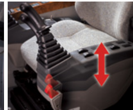
Control stand (Telescopic Function)
