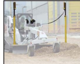
Laser control system for specially accuracy jobs leveling.
